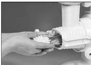
6. Slide the **Twin Gears** out.
