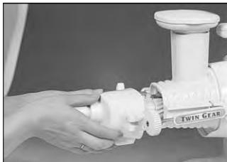
4. Slide the **Pulp Discharge Casing** over the **Twin Gear Housing**.
