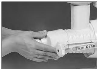
4. Remove the **Pulp Discharge Casing**.
